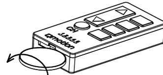
Replace the battery with a CR2032 battery. Install the battery with positive polarity side facing towards the QdR2 circuit board.
