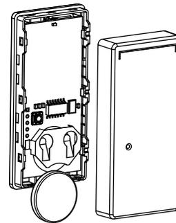
Reattach rear housing by pressing it against front housing till the snaps click into place.
